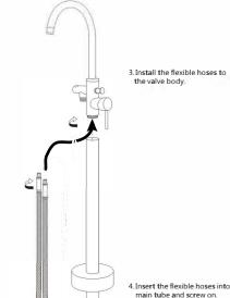
Insert the flexible hoses into the main tube and screw on.
